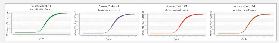
Reproducible data on four separate Azure Cielo instruments using Human GAPDH assay and SYBR Green Master Mix. Average Cg = 20.11, SD= 0.002
