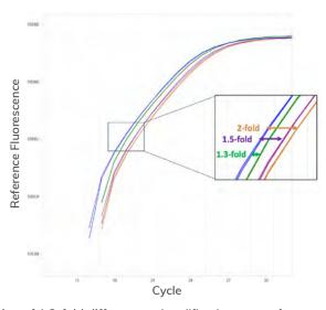
Reliable detection of 1.3-fold differences. Amplification curves for assays of GAPDH. Total human cDNA of 1.3, 1.5, and 2-fold differences in input were assessed. Assays were conducted using BioRad $^{\text{\tiny M}}$  Sso Advanced SYBR Green Mix $^{\text{\tiny 8}}$  and TaKaRa qPCR Human Reference cDNA.
